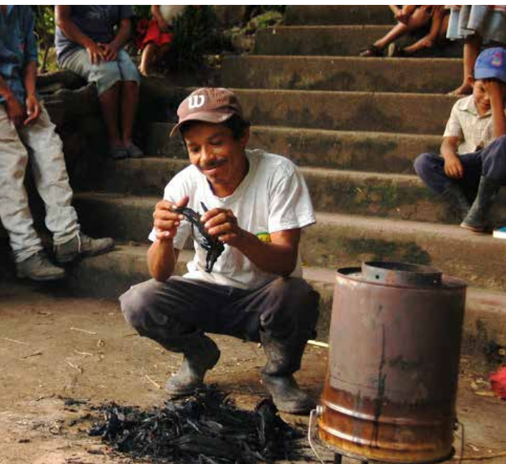
Pictured: SeaChar Estufa Finca cookstove in Nicaragua. The stove helps reduce indoor air pollution and produces biochar that can be used as a soil amendment.
