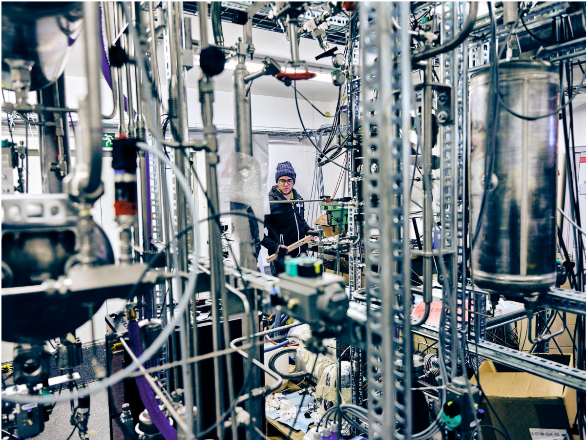
A pilot project at a Swiss university that uses Climeworks equipment to make methane out of airborne CO 2 . Luca Locatelli for The New York Times
